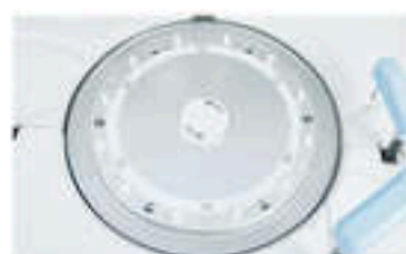
Reaction Tray 37±0.1°C, real-time monitor.
