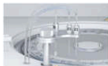
Washing Probe Independent 3-step washing system.
