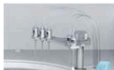
Washing Probe Independent 5-step washing system.
