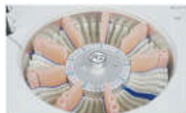
Reagent Tray 2~8°C cooling for 24 hours.
