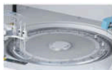
Reaction Tray 37±0.2°C, real-time monitor.
