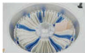
Reagent Tray 2~12°C cooling for 24 hours.
