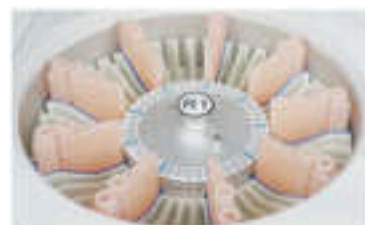
Reagent Tray 2~8°C cooling for 24 hours.
